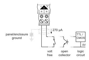
The volt free contact has a nominal wetting current of 270  $\mu A.$  The input is ON when the contact is closed.
