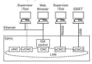
**Default CNC Addressing**: The IQ41x device (outstation) address is factory-set (in the Address module) as follows:
