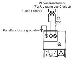
The local earth terminal (1) must be earthed (grounded) at the controller. The 24 V supply must include a suitably rated switch in close proximity and be clearly marked as the disconnecting device for the unit. Do not position the equipment so that the disconnecting device is difficult to operate.
