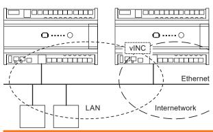
In addition, the IQ4E has the ability to join an internetwork using its virtual INC (see 'Networking' on page 4 for further details).
