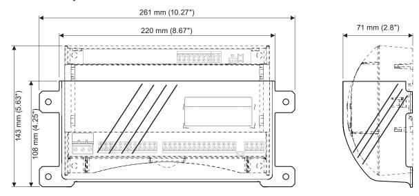
This accessory can be used with IQECO31/230, IQECO32/230 IQECO35, IQECO38 to enable the unit to comply with EN61010-1 without installation in an enclosure.
