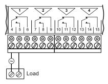
Solid State Digital Outputs (not IQECO32) (OUT5, OUT6, OUT7, OUT8)
