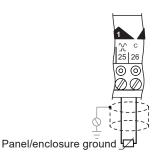
Voltage input: Used with a 0 to 10 Vdc source.
