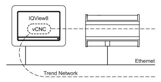
When connecting using a vCNC in another device IQVIEW8 takes the network address of that vCNC. Alarms sent to the vCNC will be received by the IQVIEW8.
