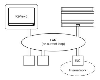
In order to join an internetwork, an INC type device (e.g. IQ4NC) will be required elsewhere on the current loop LAN.
