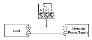
Load on when alarm not present (relay de-activated)
