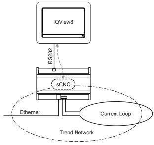
The supervisor port (sCNC) must be configured to allow network access to the Trend network.
