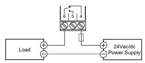
**Caution:** The relay contacts **must not** be used to switch to mains voltage; see page 11 for details of contact ratings.
