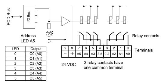
Relay energized (contact closed): LED on Relay reset (contact open): LED off 24 VDC must be connected to the +/- terminals.
