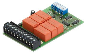
The module contains 6 relays with normally-open contacts for direct or alternating current up to 2 A, 250 VAC. The module is especially suited wherever AC switching circuits with infrequent switching have to be controlled. For space reasons, there is no integrated contact protection. Each group of 3 relays has a common connection.
