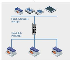
As Smart Automation Managers, PCD1.M21x0, PCD2.M5, PCD3.M2/3/5 CPUs and the programmable micro browser panel PCD7.D4xxxT5F can be used
