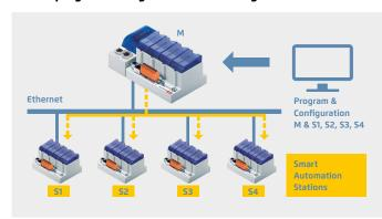
The application programs are centrally managed by the Smart Automation Manager and distributed to the Smart RIOs. If hardware is replaced, the programs and the configuration are reloaded automatically.
