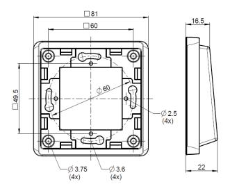
Screws shall be tighten in maximum with 0.6  $\mbox{Nm}$
