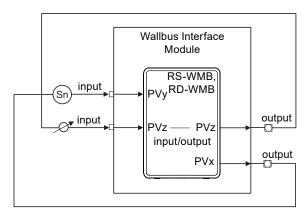
This can be seen in the diagram where PVx is the output from the RD-WMB which is connected to a sensor module in the strategy. The sensor's output is then sent back to the RD-WMB for display (PVy). This enables the strategy to change the value before display (e.g apply an offset).
