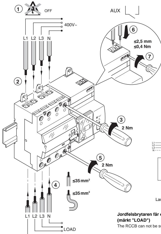
Intervention is only permitted when the unit is isolated and the device has been switched off (slide moved to the right and lever accessible)
