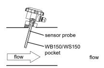
Note: The WS150 pocket is not suitable for use in a chlorine rich environment.
