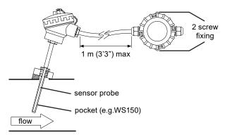
Note: The WS150 pocket is not suitable for use in a chlorine rich environment. The WB150 is not suitable for use with T-PI-160.
