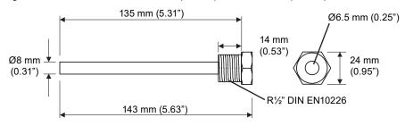
Mounting Flange (ACC/DF) for using the T-PI as duct sensor
