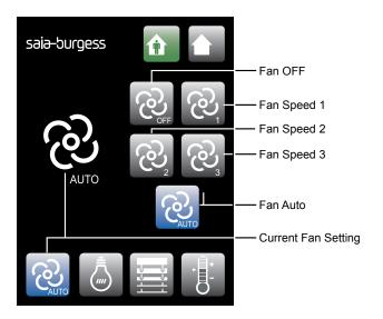
You can choose to set the fan at the speed you want (Off, 1, 2, or 3) or to follow the automatic setting (Auto) which adjusts the fan speed depending on the gap between ambient and desired temperature.
