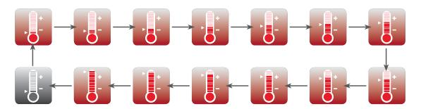
You can change the temperature setpoint by tapping the **Temperature Setpoint Status** pictogram.
