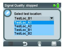
When starting a Signal Quality measurement, the currently used test location is displayed for a few seconds. By means of the menu key you may choose a different one from the downloaded list of test locations.
