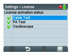
If there is already a license key for PA Test on your Tester, please provide the currently used key when ordering the Oscilloscope option. See next slide on how to retrieve the license key.
