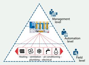
The generous memory resources (4 GByte) of the new PCD3 Power CPU make it possible to record/monitor, archive and control the data and statuses of all trades in the Saia® PCD, even without computer equipment and control system software. Applications for the various subsystems (HVAC) can be conveniently created using the graphical PG5 engineering tool and application-specific software libraries.
