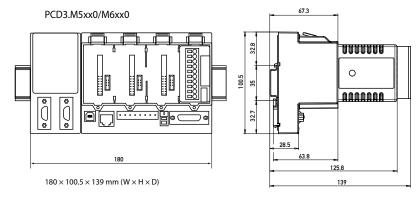
Standard and High Power CPU with slots for battery and memory modules, run/stop switch and additional interfaces
