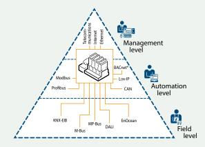
The Saia® PCD3 Power CPU has sufficient system resources to operate up to 13 communication interfaces in the same device. Even the most demanding tasks, such as simultaneous communication via BACnet® and Lon IP, are handled reliably.
