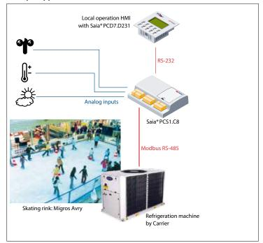
The construction and data point mix make it suitable for use in compact air conditioning devices, for example.
