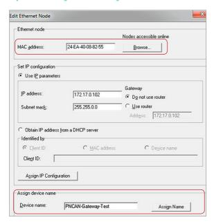
If the PN/CAN-Gateway contains the correct PROFINET name, it is recognized by the PLC and configured. When the configuration has run correctly, the blue "Mode" LED should blink.
